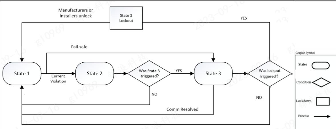
Ginlong G100 CLS was designed with a fail safe mechanism according to G100 Issue 2 2022, ensuring that in the event of communication failure or loss of source in any component, reducing the component generation to zero.
